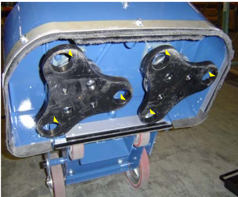
Figure 14 – Tapered Plug holders and location
