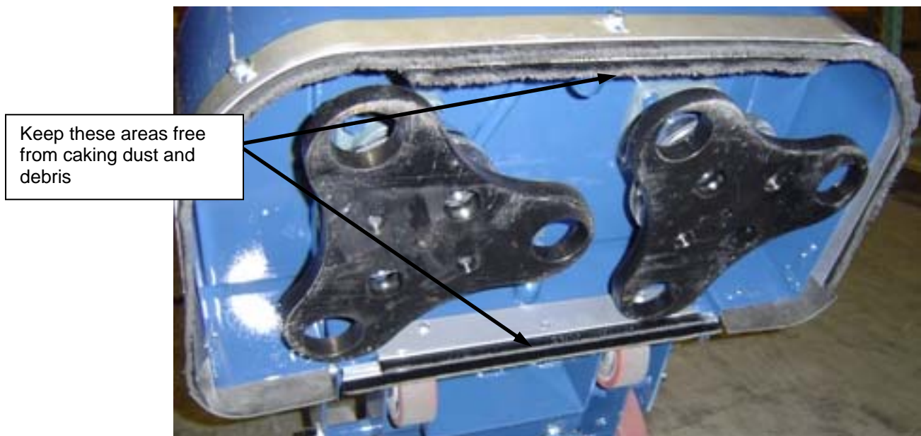
Figure 18 – Clean-out area for vacuum port
